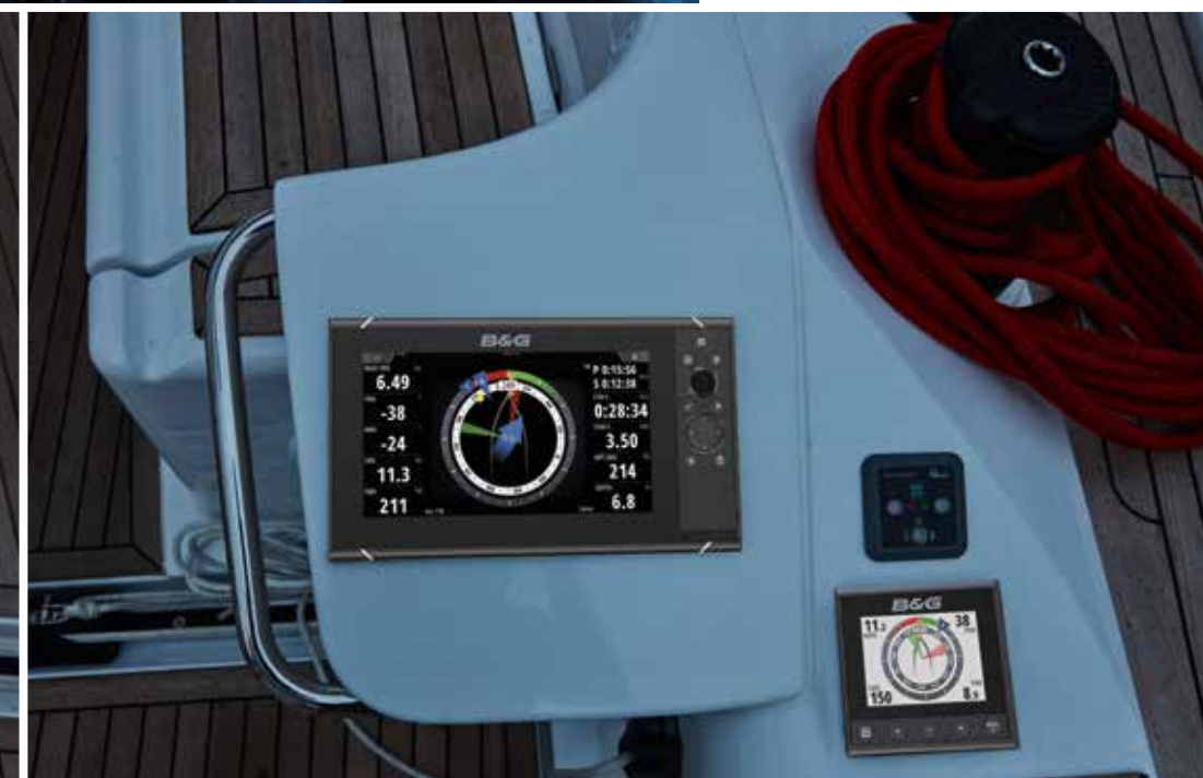
Ergonomic pod with backrest, handle and intelligent 9" multifunctional navigation display. Starboard with bow thruster control, portside with sound system.
