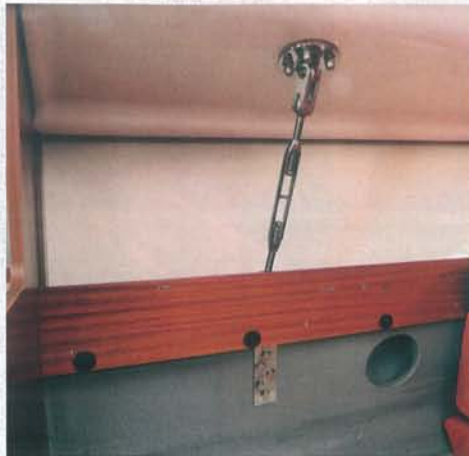
Tie-bars are attached to a return in the inner moulding that spreads the load over a large area
